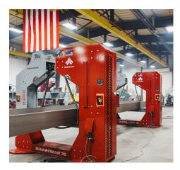
**BeamChamp®** – Allows for a more efficient and much safer way to rotate steel beams for welding and inspection applications.
